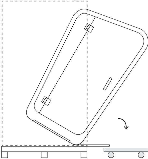
**STEP 4** Move Loop Solo to desired location on wheeled dolly.
