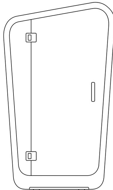
**STEP 7** Tighten all bolts on hinges to 72in/lbs torque using an alley key. Remove door straps and corner protection. Plug phone booth into wall outlet with included power cord that is located inside the booth. Enjoy!
