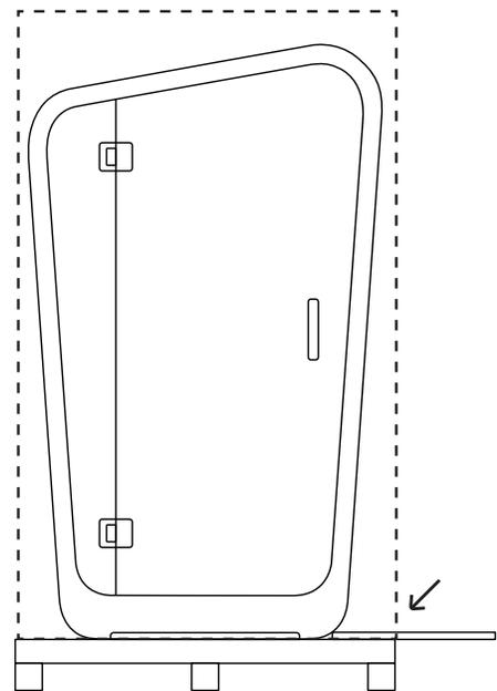
**STEP 3** Tilt booth down onto four-wheeled dolly. Confirm hinges are on top edge so that there is no risk of door swinging open.
