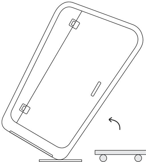
**STEP 6** Remove protective packaging and move into final location.
