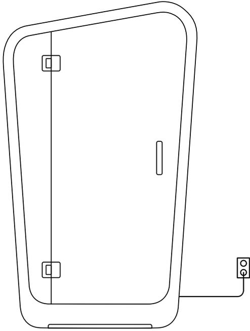
**STEP 8** Door stops come calibrated, but may be adjusted using a 9/64 allen key. Move the top and bottom adjustments in 1/4 turn adjustments until the desired magnetic grip is found.
